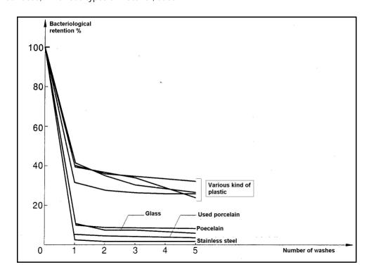
As confirmation of this fact, we should remember that there is a list of appropriate stainless steel types in the Decree of 21 March 1973, which lays down "Regulations on the hygiene of packaging, receptacles and tools intended to come into contact with substances for food use or with substances for personal use". This list numbers, with the relevant updates, around thirty types of stainless steel; definitely among those most commonly used are AISI 304 and 316 (EN 1.4301 and 1.4401).
