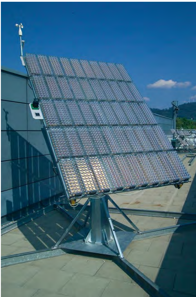
Fig. 34: Concentrating device for photovoltaic cells two-dimensionally tracked on metallic support structure (Fraunhofer ISE).
