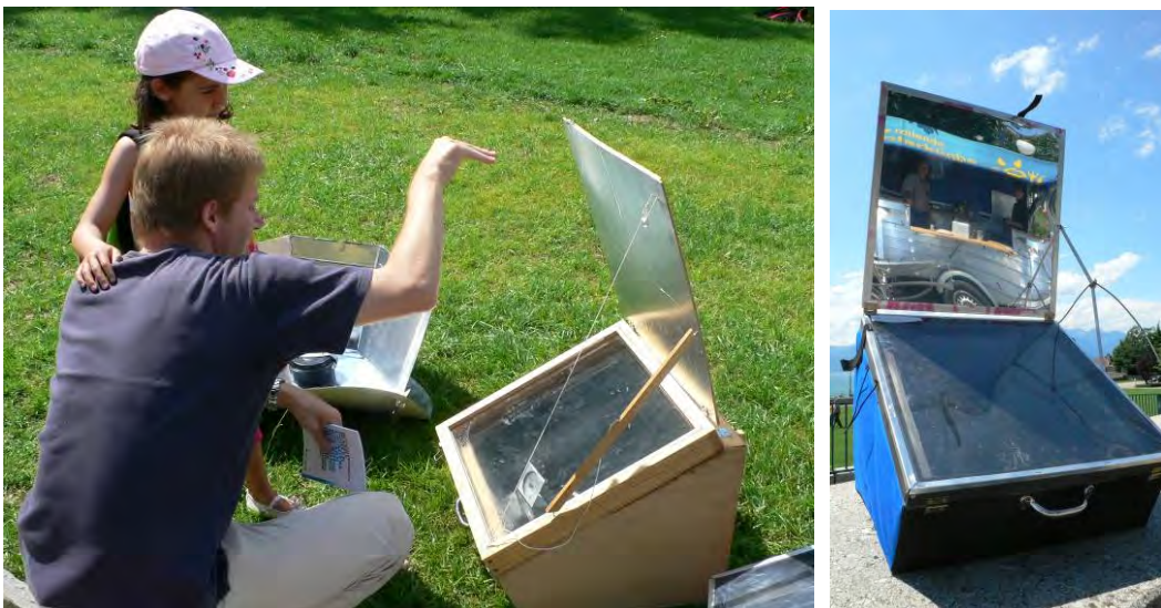
Fig. 26: Solar stoves with reflectors for better heat gain (solemyo)
