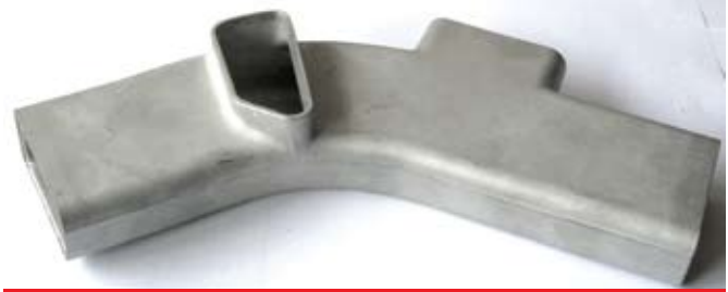
This hydroformed connecting node for an A-Pillar illustrates the high formability of stainless steels. (The original tube was rounded and straight.)
