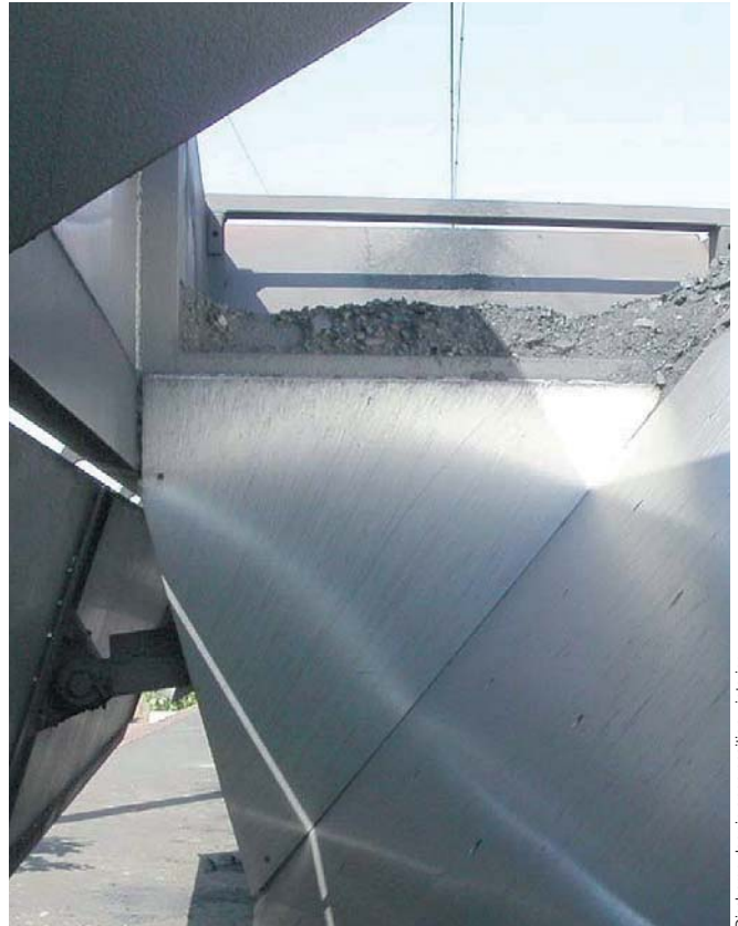
Discharge door in open position – interior.
